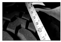
**HINT**: For example, measure from the edge of a tire tread lug to the outboard side of chassis, then repeat the measurement on other side of vehicle using <u>exact</u> same points.
