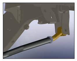
**HINT**: Bend in <u>chassis (gold) end</u> of trackbar must point <u>down</u> to prevent interference from occurring when suspension articulates.
