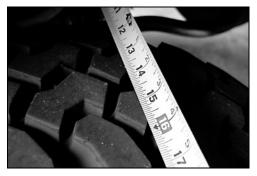
**HINT**: For example, measure from the edge of a tire tread lug to the outboard side of the chassis, then repeat the measurement on the other side of vehicle using <u>exact</u> same points.
