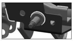
O If you are not installing a new steering stabilizer mount, plug weld Trackbar Brace to factory trackbar mounting bracket at location indicated by a "Y" in step 2.
