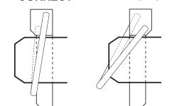
*IMPORTANT: When properly installed, the ring on the Click Pin will "snap" against the shaft of pin. When installed backwards, the ring does <u>not</u> fit snugly against shaft.*
