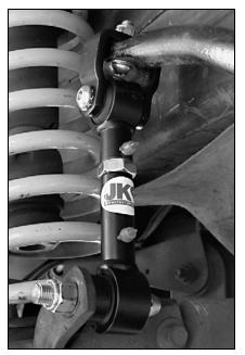
• Slide Lower End (O) of Quicker Disconnect onto the tapered Stainless Steel Posts (F).
