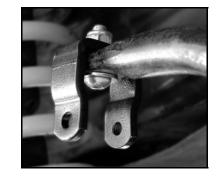
O Tighten 10mm Nylock Nut (C) to 40 ft-lb. using a torque wrench.
