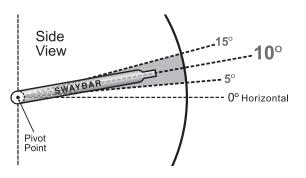
• Adjust the length of your Quicker Disconnects until swaybar is at the <u>Ideal Angle</u> or within Acceptable Range. Vehicle must be at <u>normal</u> ride height and located on <u>level</u> ground.
