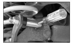
**HINT**: A small Philips head screwdriver or punch inserted into the Click Pin hole will enable you to prevent the tapered Stainless Steel Posts from rotating when tightening the Nylock nut.
