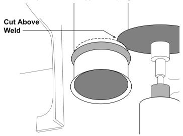
O Cut away the bump stop holder immediately above the weld as illustrated. **HINT:** A die grinder with cut-off wheel or reciprocating saw is useful for cutting away the bump stop holder.
