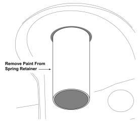
O Remove all of the factory paint from the surface of the upper spring retainer. *HINT:* Emory cloth or a suitable stripping tool is useful for paint removal.
