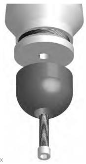
Secure the Polyurethane Bump Stop (G) to the Bump Stop Plug (F) by installing the 3/8" Flat Washer (I) and 10mm Locking Nut (J) from above the upper spring mount.
