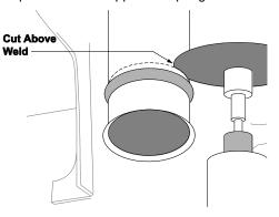
O Cut away the bump stop holder immediately above the weld as illustrated.
