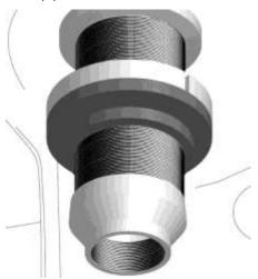
O Install Bump Shock Adapter (E) onto Threaded Tube (A) and tighten by hand until snug.
