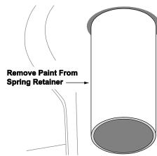
O Remove all of the factory paint from the surface of the upper spring retainer.
