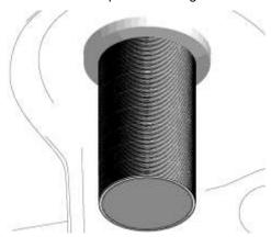
To prevent the Threaded Tube (A) from pulling away from the upper spring mount when the suspension is unloaded, the flange must be welded in place
