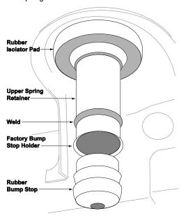
O Locate the factory weld that secures the bump stop holder to the upper coil spring retainer.
