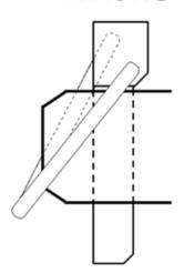
Important: When properly installed, the ring on the Click Pin will "snap" against the shaft of pin. When installed backwards, the ring does not fit snugly against shaft.
