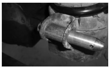
O Thread the tapered Stainless Steel Post (C) on to the 1/2" x 2-1/2" Bolt (K) from the outboard side of U-bracket and and tighten to 65 ft-lb. using a
