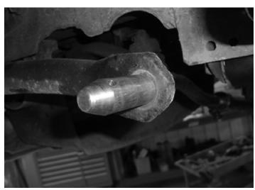
O Apply medium strength threadlocker to the tip of 1/2" x 1-1/4" Bolt (A).
