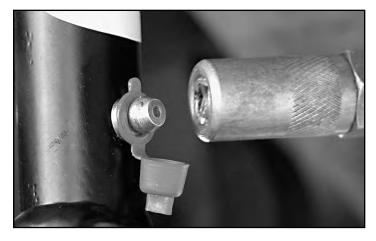
It is important to lubricate Quicker Disconnects frequently for the first three (3) months after installation to evacuate contaminants that may build up during break-in period.
