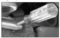
HINT: A small Philips head screwdriver or punch inserted into the Click Pin hole will enable you to prevent the tapered Stainless Steel Post from rotating when tightening the mounting bolt.
