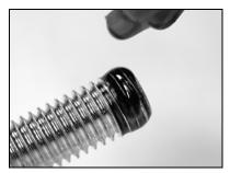
Secure tapered post to swaybar by inserting the 1/2" x 1-1/4" Bolt (A) and 1/2" Lock Washer (I) from the <u>inboard</u> side and tighten to 65 ft-lb. using a torque wrench.
