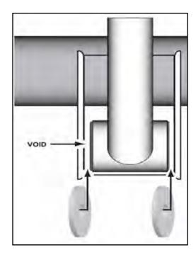
IMPORTANT: Each Control Arm requires (4) shim washers for installation. (2) 1/8" thick shim washers are required for the chassis end of the Control Arm, and (2) 1/4" thick shim washers are required for the axle end.
