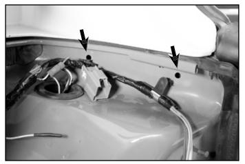
O Locate the white-tan wire that powers the 3rd brake light. Cut this wire about 4in from where it meets the main harness. Place the heat shrink wire cap over the end of the wire still part of the harness and using a heat gun or lighter seal it. Strip the lead of the remaining wire that routes back to the tailgate.
