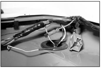
O Check to see if the factory harness includes wire taps near the plug for the 3rd brake light. If so these can be used in conjunction with the male spade terminals on the light for easy connection.
