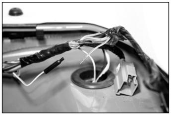
O Locate the white-violet wire running from the right tail lamp. Insert this wire into the posi-tap connector and tighten. Insert the stripped lead from the end of the white-tan wire and tighten the cap of the posi-tap connector.
