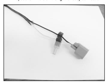
O If wire taps are not available, cut this harness before the plug and install the female wire terminals to the black and white-orange wire.
