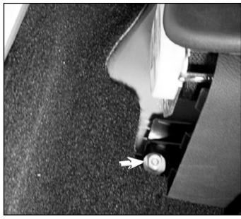
O Pull back the carpet to expose the wire harness and remove the 2 plastic clips to make the harness easier to work on.
