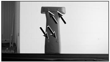
• Remove the spare tire mounting bracket from the tailgate by removing the 8 bolts using a 13mm socket.
