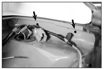
• Locate the white with tan stripe wire that powers the 3rd brake light. Cut this wire about 4 in from where it meets the main harness. Place the heat shrink wire cap over the end of the wire going forward use a heat gun or lighter seal it. Strip the lead of the remaining wire that routes back to the tailgate.
