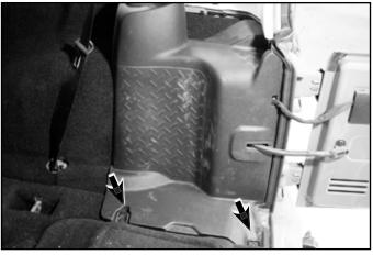
• Lastly, remove the nut located in front of seat belt to remove the inner plastic cover
