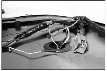
• Cut the harness near the plug for the 3rd brake light. Strip the wires and install the provided female spade terminals to the ends of the black and white-orange wire.
