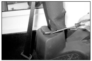
• Pull on the outside cover to release the clips and remove it.
