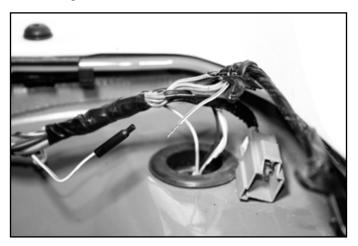
• Locate the white with violet stripe wire running from the right tail lamp. Insert this wire into the posi-tap connector and tighten. Insert the stripped lead from the end of the white-tan wire and tighten the cap of the posi-tap connector.
