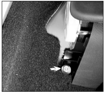
• Pull back the carpet to expose the wire harness and remove the 2 plastic clips to make the harness easier to work on.
