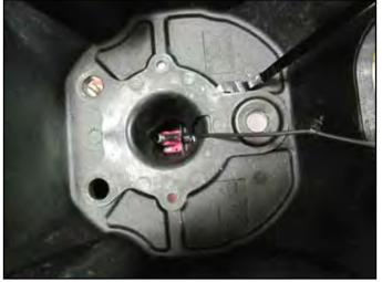
• Once the camera mount is removed remove the 3 camaera screws T8 and disonnect the camera.
