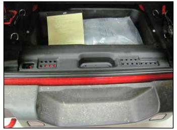
• Remove the passenger side tie down panel. Pry up the tab with a body clip tool. Then remove the bolt using a T40 bit on all 3 tie downs.
