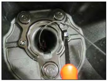
• Using a body clip tool or other appropriate tools pry the camera brack off of the spare tire mount.
