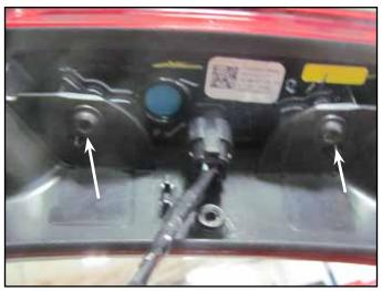
• Remove the eight bolts holding on the spare tire mount.
