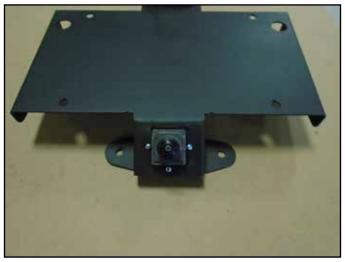
Using the provided #8-32 machine screw and nut mount the new license plate light onto the top of the lincese plate bracket. Phillips screwdriver and 11/16 socket/wrench. Torque to 18 in-lbs
