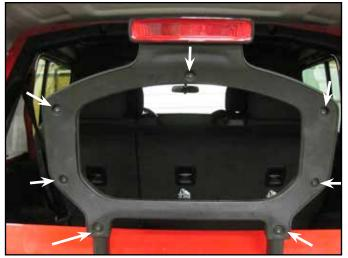
• Remove and unplug the 3rd brake light by removing the two T25 screws.
