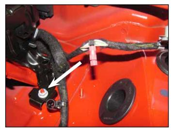
• Locate the provided wire. Strip both strands of wire on one end. Attach the red wire strand to the other end of the posi tap. Also crimp the ring terminal to the black wire strand. Place the ring terminal onto the seat belt bracket stud and tighten down the OE flange nut
