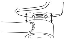
IMPORTANT: The Chassis End of Adjustable Trackbar must be in the "neutral" position (as illustrated above) before the Jam Nut is tightened.
