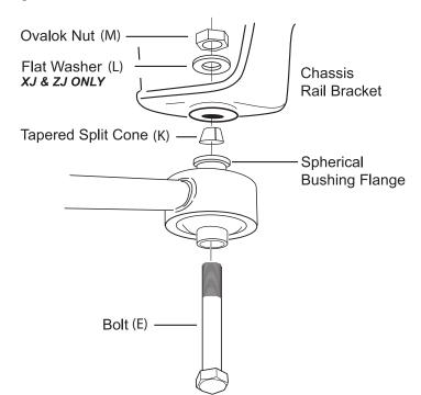
**HINT:** Tapered Split Cone (K) should be located between flange of spherical bushing (G) and mounting surface of chassis rail bracket, with the narrow end of tapered cone facing up towards chassis.
