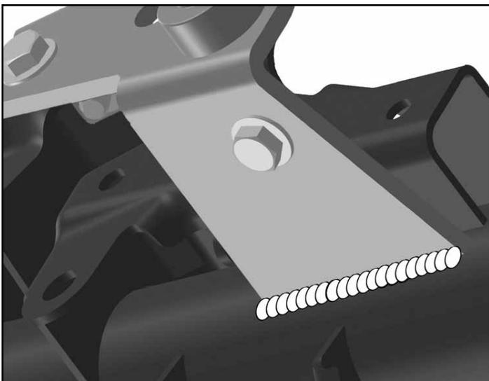
**IMPORTANT: Avoid overheating axle tube and factory track bar bracket by welding a small section and allowing the surface to cool off regularly.**
