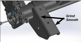
O Measure down from the factory lower control arm hole 1-3/8" and mark a horizontal line. Trim and remove this section from the vehicle.
