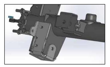
O Once the bracket fitment has been verified, remove bracket and coat area with paint.
