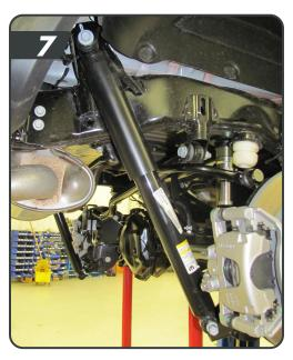
Lower the axle enough to remove the factory springs. Note the orientation of the upper spring isolators. Make sure there is adequate slack on all brake lines.
