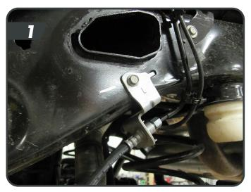
Remove the (2) bolts holding the TPMS ECU sensor to the rear crossmember (10mm) [2].
