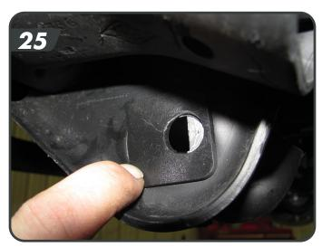
Re-install the control arm to the axle with the factory bolt with cam lock washers. Rotate the cam lock so that the bolt will be as far back in the slot as possible (most rearward setting = max caster). [26] Snug the cam hardware so that the cams are retained within the stops. Final torque will be completed with the weight of the vehicle on the suspension.
