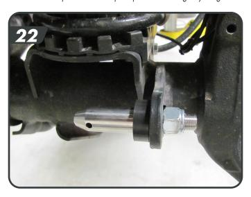
The kit comes with disconnect retention brackets to hold the links when the links are disconnected. Install the retention brackets using the provided 5/16" bolts into the factory hole in the front of the coil bucket [23]. These are designed to slightly interfere with the edge of the coil bucket to hold them in place.
