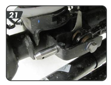
m. Install the longer disconnect post on the driver side axle sway bar link mount with it pointing inboard [22]. Fasten with the ½" nylock nut and tighten to 64 ft-lbs. Tighten the post with the pin hole parallel to the ground. Slide the polyurethane spacer on the pin up against the axle tab.
