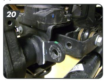
Install the shorter passenger side post on the side of the track bar mount at the sway bar link mount location with it pointing outboard [21]. Fasten with the ½" nylock nut and tighten to 64 ft-lbs.
