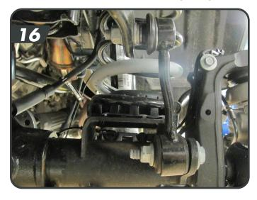
Remove the 4 bolts mounting the front driveshaft to the pinion flange (15mm). This is done to ensure the driveshaft does not bind when removing the coil springs. [17]
