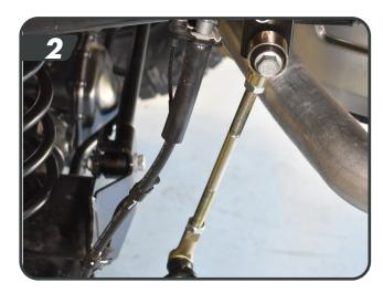
Install the rear bump stop spacers on the axle. Fasten the bump stop spacer to the axle with the 5/16" x 7/8" bolts, nuts and washers. Torque bolts to 20 ft-lbs. (½") [3]
