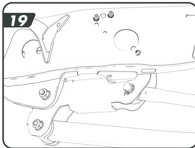
**Note:** it may be easier to align the control arms to the mount by removing the opposite side upper control arm and adjusting the axle with a hydraulic jack.
