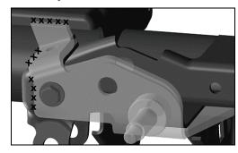
**HINT:** Be sure to include area on factory coil spring bracket and lower base of Relocation Bracket where it terminates just before it makes contact with axle tube.
