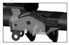
With the Relocation Bracket (A) in position, insert one 3/8" x 1" GR5 Bolt (B) with Flat Washer (C) into original mounting hole as illustrated below. Secure bolt with another 3/8" Flat Washer (C) and Ovalok Nut (D) and temporarily tighten to hold the bracket securely to the factory axle housing bracket.
