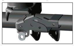
Position the Relocation Bracket (A) against the factory track bar bracket as illustrated.
