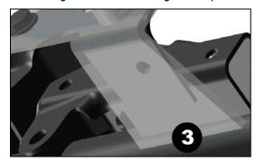
Next, fillet weld Steering Stabilizer Relocation Bracket (A) to axle housing at all locations indicated by an "X" in step 2.
