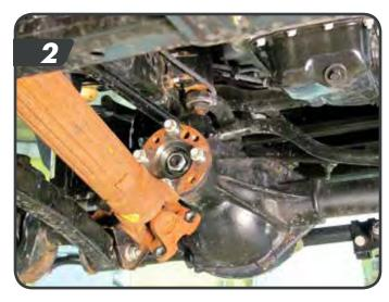
Disconnect the steering drag link from the pitman arm to ensure it doesn't bind when installing the new coil springs. Remove the tie rod end nut and dislodge the tie rod end from the pitman arm. Save nut. [3]
