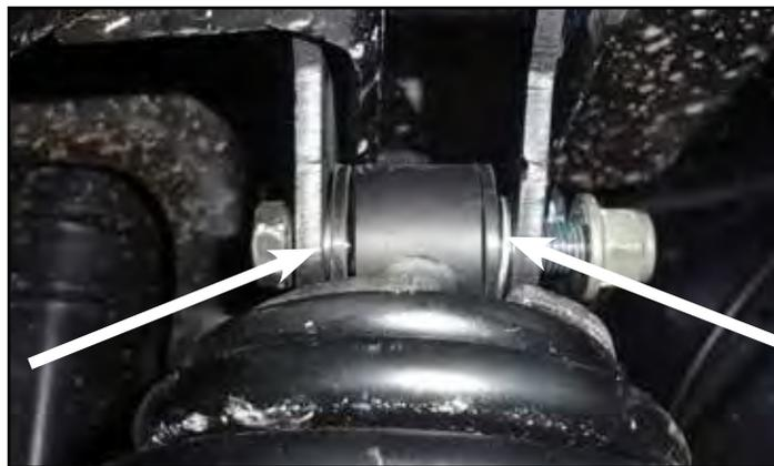
10. Tighten all three fasteners to 40 ft-lbs.
