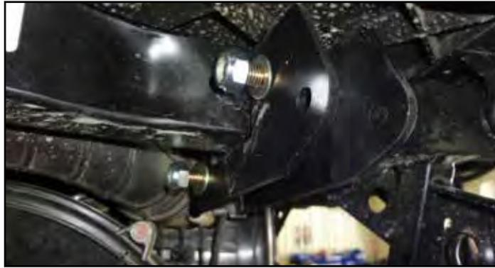
22. Install the shock to the new lower mount with the factory hardware.
