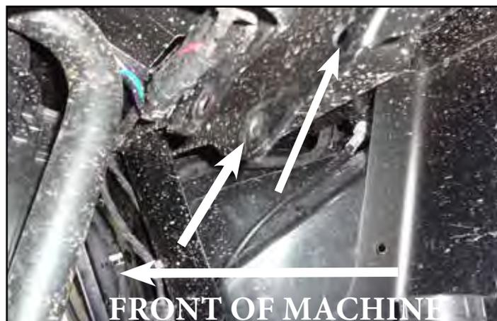
7. Insert a 04056 spacer sleeve through the two bolts and followed by another front lift bracket.
