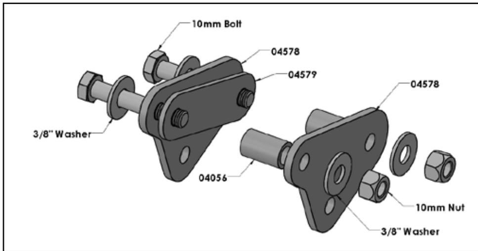
5. Insert two 10mm bolts and 3/8" washers through the two upper holes in the front lift bracket (04578), followed by a front lift bracket spacer (04579). The spacer is included to space the lift bracket off the surface because of the flange on the factory upper shock mount.
