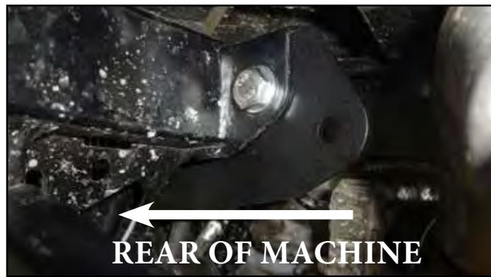
20. Install another rear lift bracket on the outside of the factory shock mounts onto the 10mm bolts.
