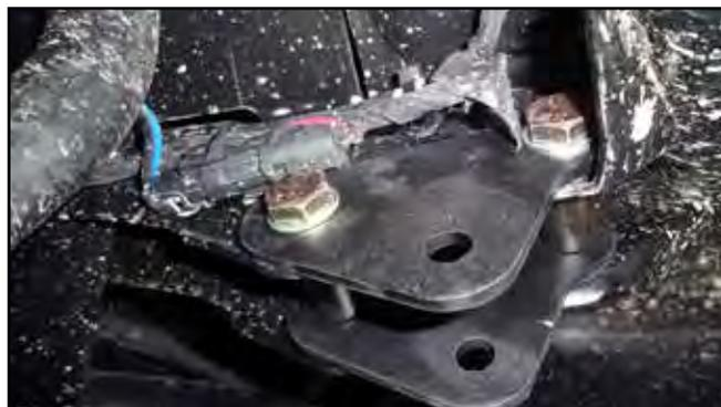
8. Install a 3/8" washer and 10mm nut to the back side of the two bolts.
