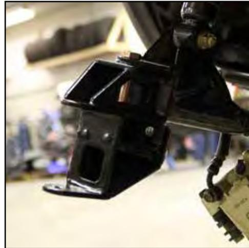
9. Once the holes are drilled, install and tighten the supplied 3/8" bolts. Once the bracing bolts are tightened, finish tightening the OEM spindle bolts. The torque for these should be around 60 ft./lbs.
