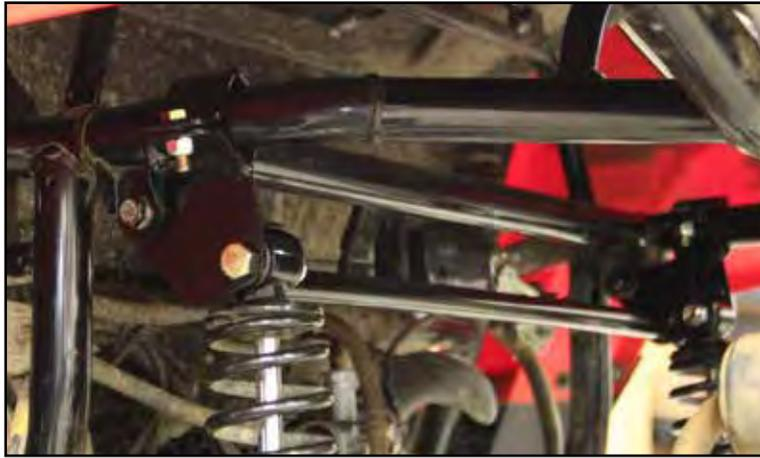
23. Use the supplied clamps and 5/16" hardware to install the clamps over the chassis tube and secure the relocater in place.
