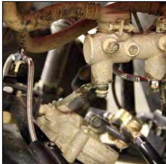
13. Once the new lines are installed and tightened, bleed the brakes thoroughly.
