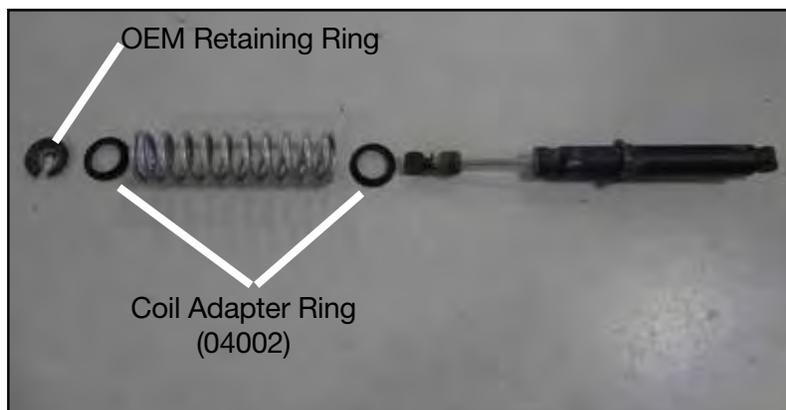
3. Compress the new spring enough to fit another coil adapter ring (04002) and the OEM retaining ring. Make sure the preload adjuster is all the way down to allow for the easiest installation.
