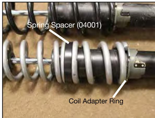
6. Make sure a coil adapter ring is installed on the end of the short spring contacting the preload adjuster ring as well as on the end of the long spring contacting the OEM retainer.
