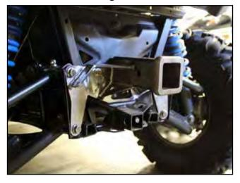
Slide included spacers between the hitch reciever and frame and install included 5/16" Bolts, Nuts and 1/4" washers. See Figure 2.
