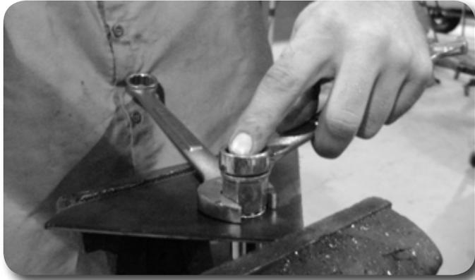
Figure 2 - 1/2" Rivet Nut shown
