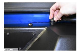
14. INSTALL 2 BOLTS AND NUTS ON BOTH SIDES OF THE BUMPER. DO NOT TIGHTEN FIG. 33
