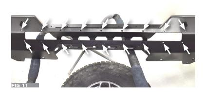
3. INSTALL THE SHORT BUMPER TRIM PLATE TO THE FRONT OF THE BUMPER USING THE PROVIDED 13 BOLTS AND NUTS. NO NOT TIGHTEN UNTIL ALL HARDWARE IS INSTALLED. FIG. 12
