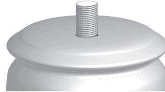
**IMPORTANT:** Do NOT thread 1/2" x 2" Stud more than one inch into the 2.00" spacer.
