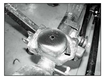
• Place the provided bump stop extension inside one of the coil springs. Re-install the coil springs with the bump stop extension inside. Make sure the spring is seated properly in the axle mount.
