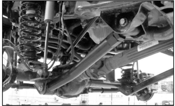
**HINT:** If mounting bolt is difficult to install due to misalignment of Control Arm bushing with mounting bracket, either (1) adjust height of axle housing with hydraulic jack, (2) move axle housing into position with a heavy-duty ratchet strap, or (3) temporarily disconnect track bar until mounting holes align.
