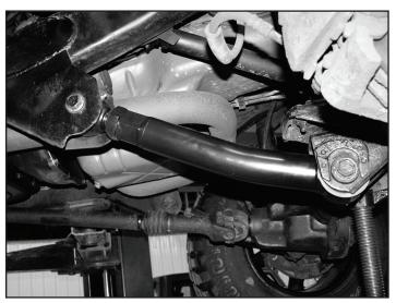
Install the original mounting bolt and finger tighten the nut. Remember to realign cam adjuster on front axle if equipped. DO NOT torque mounting hardware until instructed.
