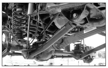
HINT: If mounting bolt is difficult to install due to misalignment of Control Arm bushing with mounting bracket, either (1) adjust height of axle housing with hydraulic jack, (2) move axle housing into position with a heavy-duty ratchet strap, or (3) temporarily disconnect track bar until mounting holes align.
