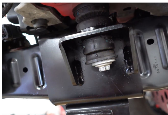
High Clearance Body Mount - Installed
