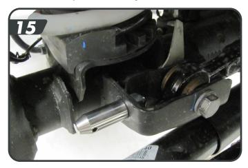
r. Install the longer disconnect post on the driver side axle sway bar link mount with it pointing inboard [16]. Fasten with the ½" nylock nut and tighten to 65 ft-lbs. Tighten the post with the pin hole parallel to the ground. Slide the polyurethane spacer on the pin up against the axle tab.
