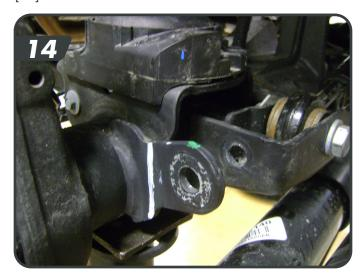
q. Install the shorter passenger side post on the side of the track bar mount at the sway bar link mount location with it pointing outboard [15]. Fasten with the ½" nylock nut and tighten to 64 ft-lbs.
