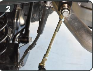
Install the rear bump stop spacers on the axle. Fasten the bump stop spacer to the axle with the  $5/16" \times 7/8"$  bolts, nuts and washers. Torque bolts to 20 ft-lbs. (1/2") [3] - 3" extension shown]
