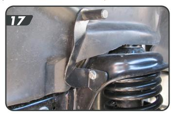
t. JT Mojave models with JKS9613: Install two provided ½" donut spacers (01499) between the reservoir hose retaining wire and frame using the OE bolt [18] and tighten to 6 ft-lbs (first mount forwards of the coil spring). Verify reservoir hose clearance to the disconnect retention bracket once installed.
