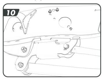
Note: It may be easier to align the control arms to the mount by removing the opposite side upper control arm and adjusting the axle with a hydraulic
