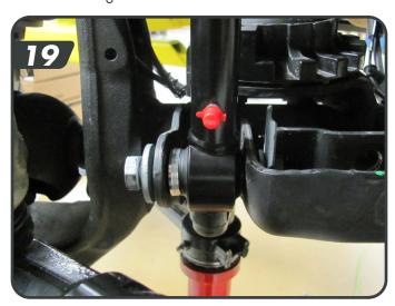
aa. Install the remaning longer sleeve on the driver side and slide the polyurethane spacer onto the sleeve so it will mount towards the axle mount tab. Install the quicker disconnect to the inboard side of the axle tab with the original sway bar link hardware.
