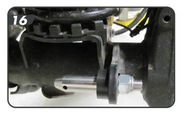
s. The kit comes with disconnect retention brackets to hold the links when the links are disconnected. Install the retention brackets using the provided 5/16" bolts into the factory hole in the front of the coil bucket [17]. These are designed to slightly interfere with the edge of the coil bucket to hold them in place.
