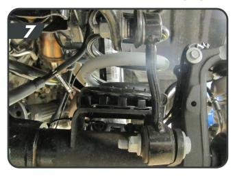
Remove the 4 bolts mounting the front driveshaft to the pinion flange (15mm). This is done to ensure the driveshaft does not bind when removing the coil springs. [8]
