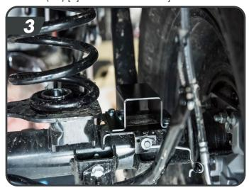
d. The shocks come with the bushings and upper spacers pre-installed. JSPEC shocks will be installed body down, Fox shocks will be installed body up. Slide the shock up into the mount.
