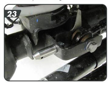
r. Install the longer disconnect post on the driver side axle sway bar link mount with it pointing inboard [24]. Fasten with the ½" nylock nut and tighten to 64 ft-lbs. Tighten the post with the pin hole parallel to the ground. Slide the polyurethane spacer on the pin up against the axle tab.
