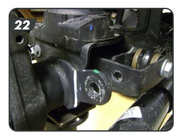
q. Install the shorter passenger side post on the side of the track bar mount at the sway bar link mount location with it pointing outboard [23]. Fasten with the ½" nylock nut and tighten to 64 ft-lbs.
