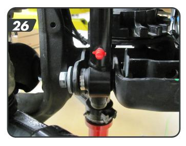
z. Install the remaning longer sleeve on the driver side and slide the polyurethane spacer onto the sleeve so it will mount towards the axle mount tab. Install the quicker disconnect to the inboard side of the axle tab with the original sway bar link hardware.
