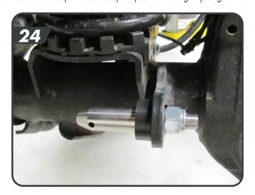
s. The kit comes with disconnect retention brackets to hold the links when the links are disconnected. Install the retention brackets using the provided 5/16" bolts into the factory hole in the front of the coil bucket [25]. These are designed to slightly interfere with the edge of the coil bucket to hold them in place.
