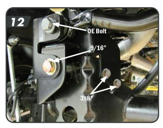
q. Drill the holes and fasten the bracket to the axle with the provided hardware. Insert the provided sleeve in the OE track bar position.
