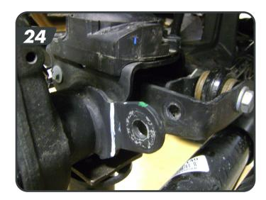
t. Install the shorter passenger side post on the side of the track bar mount at the sway bar link mount location with it pointing outboard [25]. Fasten with the ½" nylock nut and tighten to 64 ft-lbs.
