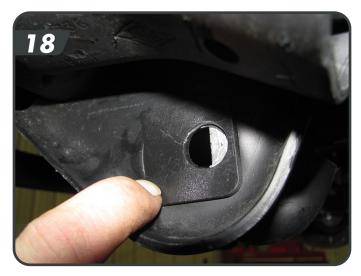
d. Re-install the control arm to the axle with the factory bolt with cam lock washers. Rotate the cam lock so that the bolt will be as far back in the slot as possible (most rearward setting = max caster). Snug the cam hardware so that the cams are retained within the stops. Final torque will be completed with the weight of the vehicle on the suspension. [19]
