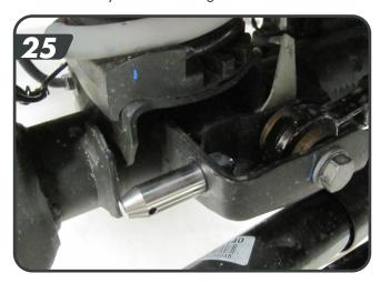
u. Install the longer disconnect post on the driver side axle sway bar link mount with it pointing inboard [26]. Fasten with the ½" nylock nut and tighten to 64 ft-lbs. Tighten the post with the pin hole parallel to the ground. Slide the polyurethane spacer on the pin up against the axle tab.
