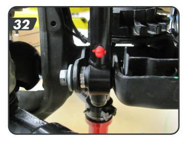
aw. Install the remaning longer sleeve on the driver side and slide the polyurethane spacer onto the sleeve so it will mount towards the axle mount tab. Install the quicker disconnect to the inboard side of the axle tab with the original sway bar link hardware.
