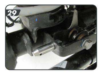
ao. Install the longer disconnect post on the driver side axle sway bar link mount with it pointing inboard [30]. Fasten with the ½" nylock nut and tighten to 64 ft-lbs. Tighten the post with the pin hole parallel to the ground. Slide the polyurethane spacer on the pin up against the axle tab.
