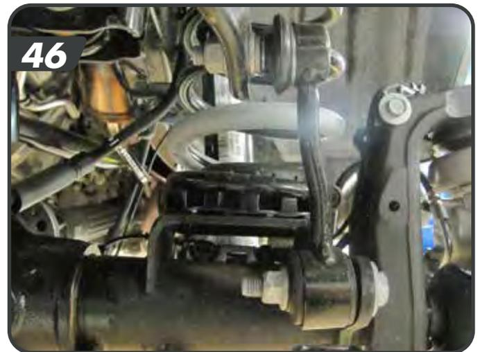
i. Remove the 4 bolts mounting the front driveshaft to the pinion flange (15mm) and support it with a strap or bungee cord. This is done to ensure the driveshaft does not bind when removing the coil springs. [47]
