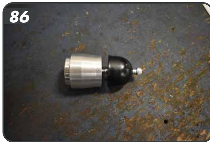
t. Place loctite on the bolts threads and insert the assembly into the bottom of the bump stop tube on the front coilover frame bracket.
