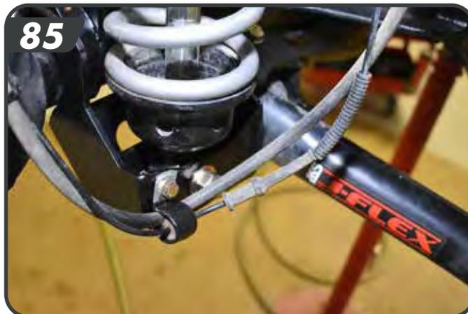
m. Reattach the factory brake line to the frame through the frame mount with OE hardware (10mm). Torque Bolt to 115 in-lbs.
