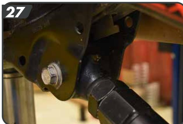
**HINT:** If mounting bolt is difficult to install due to misalignment of the control arm bushing with mounting bracket, either (1) adjust height of axle housing with hydraulic jack, or (2) move axle housing into position with a heavy-duty ratchet strap.
