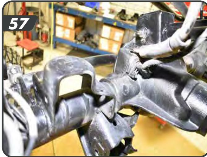
e. Using a cut off wheel cut the LCA mount flange of the axle as shown. [58]
