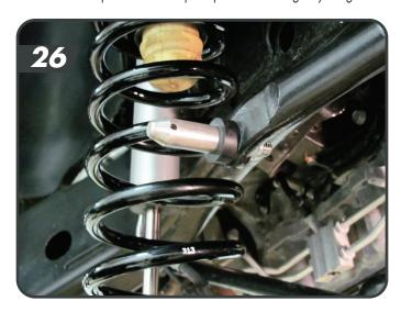
Remove the nut an install the lower mounting posts into the factory sway bar link holes so they are pointing inboard and the pin holes are parallel to the ground. The passenger side post is squared off to provide clearance between the post and the OE track bar bracket. [27]
