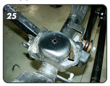
b. Place the provided bump stop extension inside one of the JSPEC front coil springs. Note: Taller springs are for the front. Install the front coil springs with the bump stop extension. Make sure the spring is seated properly in the axle mount.
