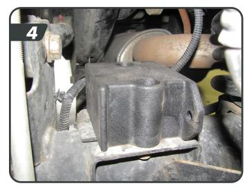
e. Install the JSPEC shocks into the vehicle with the factory hardware.
