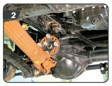
h. Disconnect the steering drag link from the pitman arm to ensure it doesn't bind when installing the new coil springs. Remove the tie rod end nut and dislodge the tie rod end from the pitman arm. Save nut. [3]
