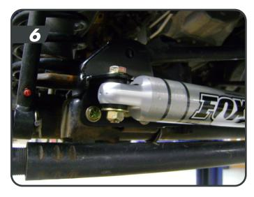
1. If using the factory steering stabilizer, use the factory axle hardware to mount it to the bracket. If an aftermarket stabilizer is installed, use the provided ½" bolt, nut, and washers from bolt pack J110. The larger diameter washer is used on the bottom against the stabilizer bushing.
