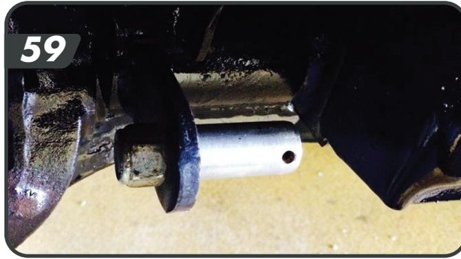
*Note: In some cases a rotary grinder may be necessary to slightly open up the sway bar hole to clear the 1/2" bolt. This ensures a tight fit.*
