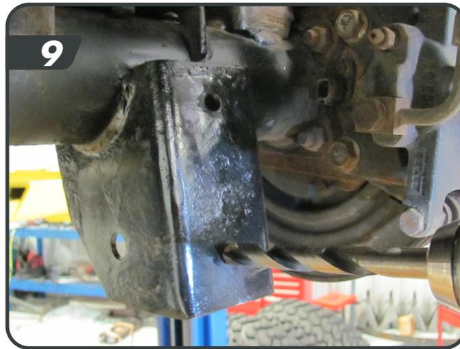
d. Place the JKS lower coilover mount over the factory bracket. Line the bracket up by temporarily installing the factory control arm bolt and line up the 2 rear holes. Use the provided 7/16" hardware to attach the bracket to the mount. The flange lock nuts can be placed on the bolts using a magnet from the top. Tighten hardware to to 70 ft lbs [11].
