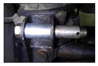
• Tighten the 1/2"-20 x 2-1/2" bolt to 65 ft-lb using a torque wrench.
