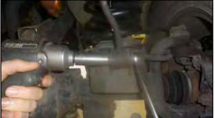
After both links are disconnected from the axle, pull down on the sway bar to gain access to the bolts to disconnect the sway bar links from the sway bar (18mm). If links are after market, measure eye-eye length. If they are longer than 9-3/4", see "Important Notes". Discard links and Hardware
