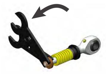
• Slide the spring off of the shaft.
