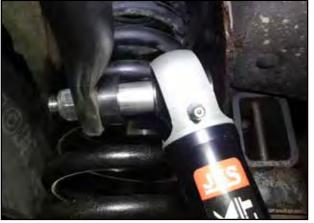
• Push the sway bar back up and slide the lower end of the Flex Connect on both the driver and passenger sides onto the tapered Stainless Steel Posts
