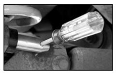
*Hint*: A small Phillips head screwdriver or punch inserted into the Click Pin hole will enable you to prevent the mounting post from rotating when tightening the nut.
