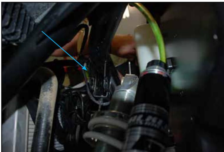
7. When installing the lift bracket make sure the bracket with the “U” shape goes behind the front factory shock mounts and frame facing upward.
