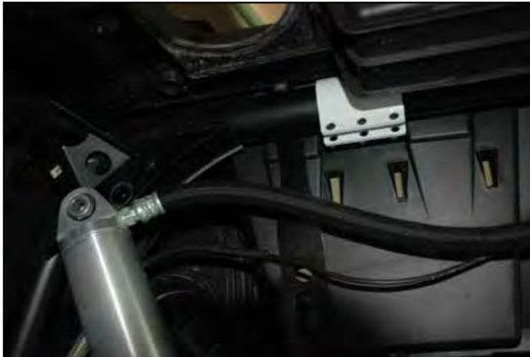
18. Next install the rear lift bracket itself into the horizontal frame bracket aligning all three holes and loosely installing the (3) three allen head bolts and nuts. At the same time install the front of the bracket into the factory frame shock mount.
