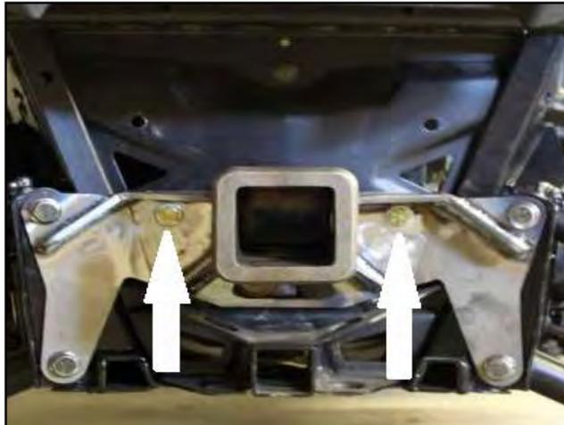
6. Torque 5/16" hardware to 24 ft-lbs, Torque control arm bolts to 40 ft-lbs.
