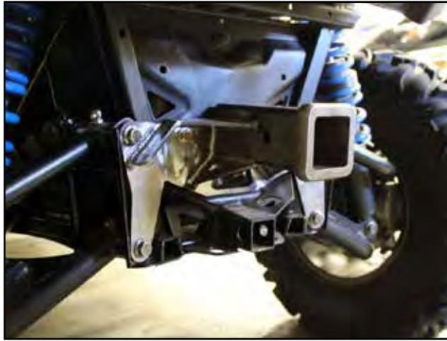
5. Slide included spacers between the hitch receiver and frame and install included 5/16" Bolts, Nuts and 1/4" washers. See Figure 2.
